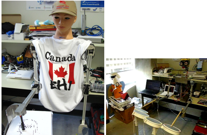
Fig. 7. BETTY: Upper body and face robot acting as portrait artist and drummer
