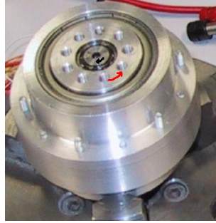
Fig. 3. ARCHIE: Modular Joint Design combining a brushless motor and a harmonic gearbox
