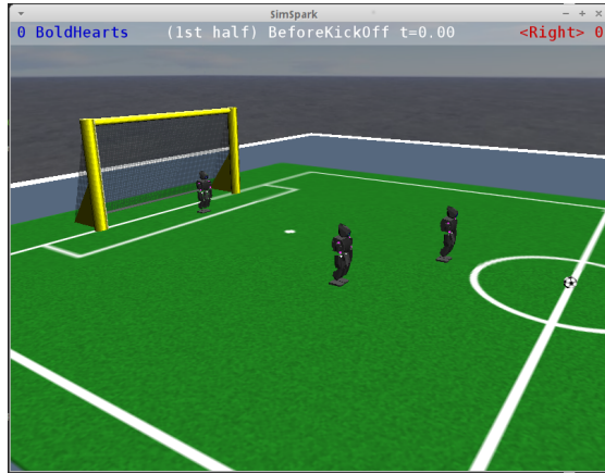
Fig. 2. SimSpark based simulation of DARwIn-OPs in a kid-size field.
