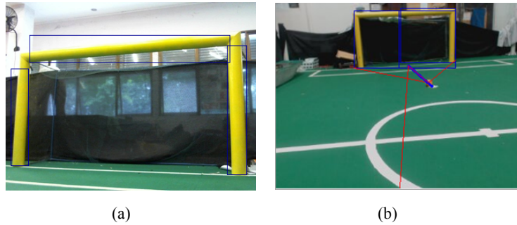
Figure 9. Object segmentation and identification of goal on the field
