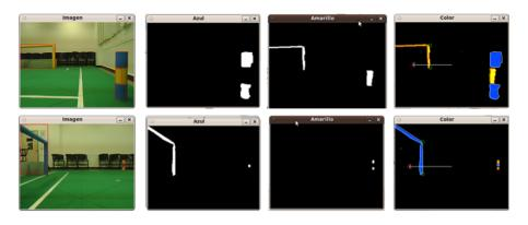
Figure 4. Two different cases showing the process to seek for the opposite goal and beacons.
