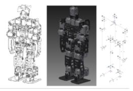
Figure 3. Kinematic diagram of the DARwIn-OP based prototype.
