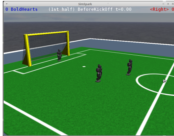
Fig. 2. Simulation of a team of DARwIn-OPs in a kid-size field, implemented on the RoboCup soccer simulator
