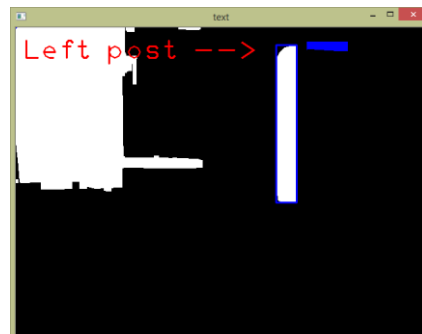
(b) The crossbar is detected (colored in blue), and the algorithm detects that the post in the image is the left post.
