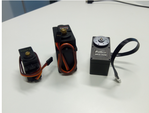
Fig. 4. Left: MG995, Center: FeeTech FS6535, Right: FeeTech SM30.
