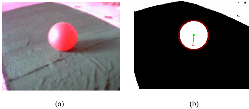
Fig 4: (a) the placement of the ball on the field. (b) the detected ball on the field using circular hough transform.
