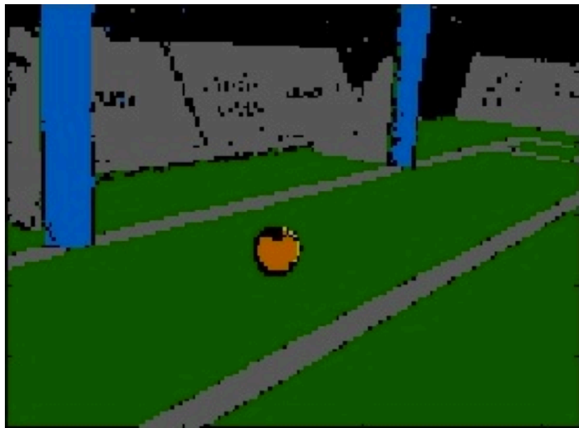
Fig. 5. Visualization of the color segmentation
