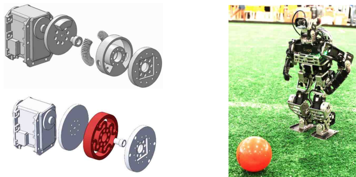
Fig. 1: Top left: first version of our modular Series Elastic Actuator. Bottom left: work-in-progress simplifying the design, now we are simplifying even further to only two moving parts. Right: Kid Size Humanoid from WF Wolves equipped with SEAs in the knees during RoboCup 2014.
