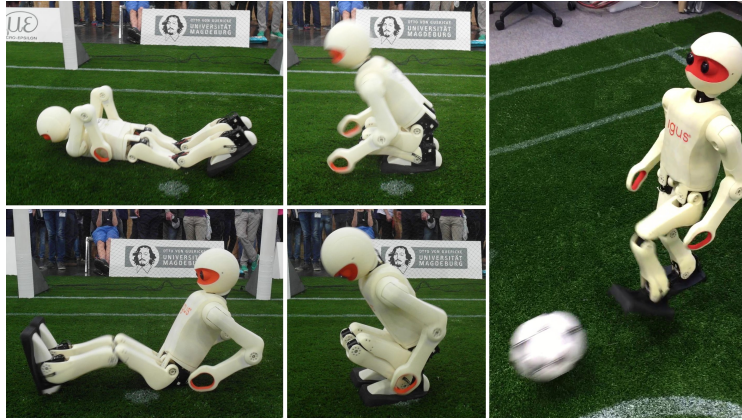
Fig. 4. Dynamic get-up motions of the igus Humanoid Open Platform, from the prone (top row) and supine (bottom row) lying positions, and a still image of the kick motion.
