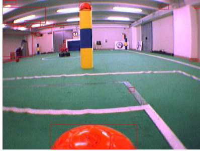
Fig. 6. Connected regions extracted from the frontal camera; some false positives are present.
