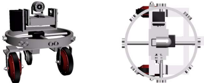
Figure 1: IVWAN's differential drive configuration: two main wheels each driven by its own motor. A third wheel is placed in the rear to passively roll along while preventing the robot from falling over.
