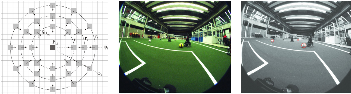
Fig. 6. Left: Principle of the ball detection algorithm. For a number of points on a circle with radius r around the pixel the derivative in the direction of the center point is calculated. The sum of these derivatives for radius r gives the confidence measure of a circle with a radius r being present at this pixel. Center: Example image from the front camera. Right: Image of the front camera with ball detection (Note that the blue ball is not detected due to the shape after the gradient operation).
