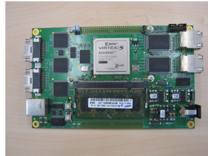
Fig. 7. Specifications and photo of the FPGA Vision Platform, designed for the goalkeeper robot.
