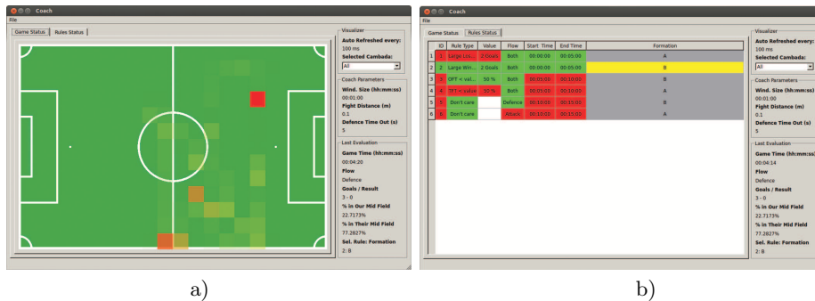
Fig. 5. Screenshots of the the coach application. a) Game status reflecting current game flow, result, percentage of time in each midfield and current formation. b) Rules status defining the current parameters and thresholds for changing ongoing strategy.
