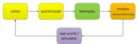
The software architecture can roughly be divided into Vision, World Model, Team Play and Motion. The Vision package of the software comprises of two main nodes that perform ball/obstacle detection and localization.
