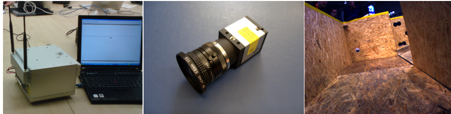
Fig. 3. Our mobile computing platform with CUDA capable GPU (left) and uEye camera (middle), and a picture taken by the camera at RoboCup German Open 2009 in Hannover (right).
