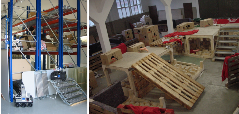
Fig. 7. Two rescue arenas available at the Jacobs University: the high bay racking system based arena (left) and the new RoboCup-like arena (right).
