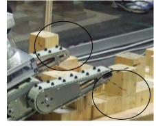
Some flexible fibers are attached at the edge of the flippers. The fiber has no advanced sensors or data connection to the operator PC, it just attached there. When the flipper is very near to the wall or obstacle, the fiber will bend and the fiber curvature indicates the distance between the flipper and the wall. The curvature can be observed through camera, so this "cat whisker" sensor gives detailed distance information around the flipper edge without complex mecha-
