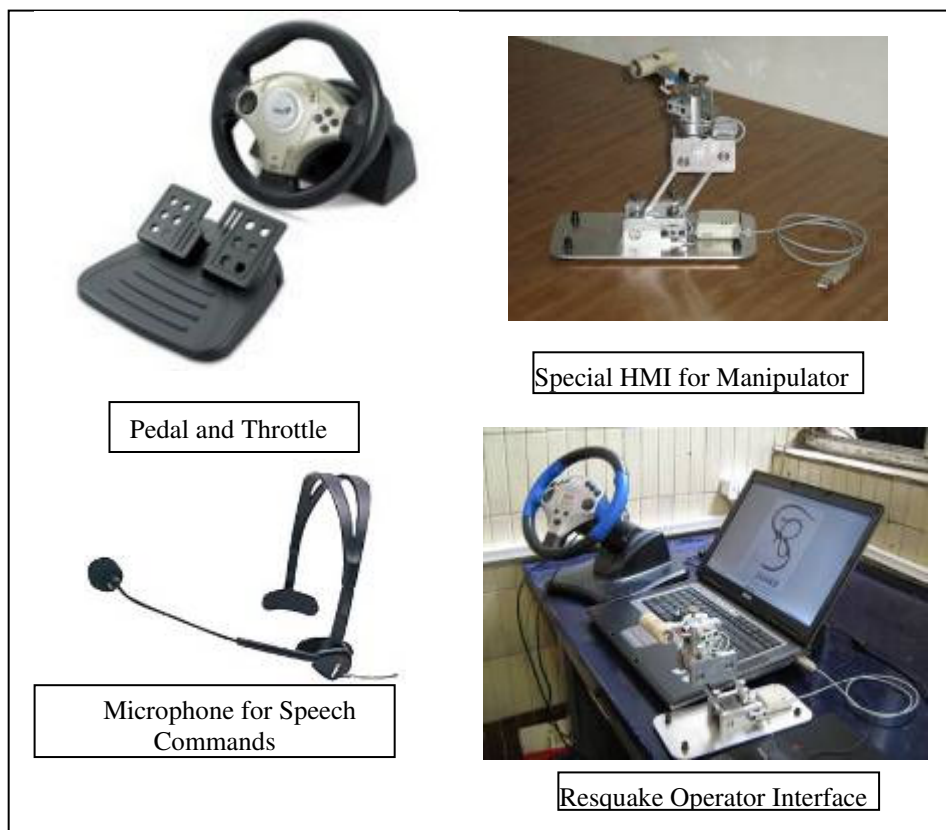
Fig 1. Operator Interface, Pedal-Throttle, Microphone and Special HMI For capturing Pedal-throttle data, we use DirectX SDK 9 and for working with microphone and create speech commands, we use Microsoft speech recognition SDK.
