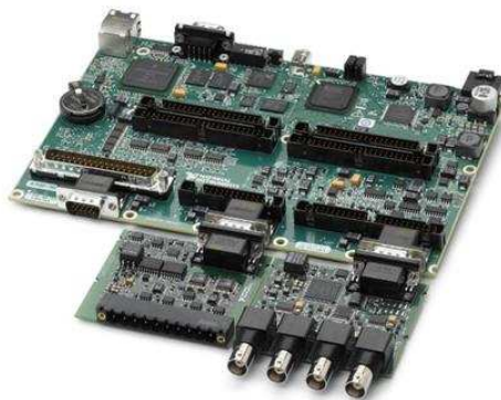
Fig. 1. Single Board RIO with a 4 Channel IEPE 1 and AC/DC Analog Input Module and a module for digital outputs
