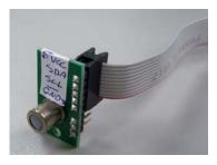
The I2C output of the sensor will be connected to the Devantech Ltd. USB to I2C Interface Module to be interpreted directly on the computer.
