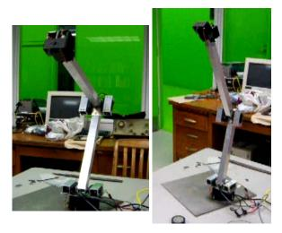
Base composed of the Lynxmotion Base Rotate Kit powered by a Hitec HS-645MG Servo Motor.
