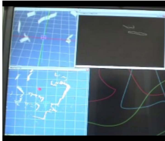
Fig. 7 human-robot interface for KAMUI. Up-left; wall image based on laser range-finder. Up-right; the area enclosed with white line is high temperature area by thermal camera. Low-left; generated 2D map of the environment.
