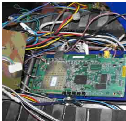
Fig. 3. Dlink Access Point Board
