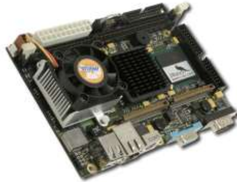
Fig 4.7 Embedded card JRex used for robot controller
