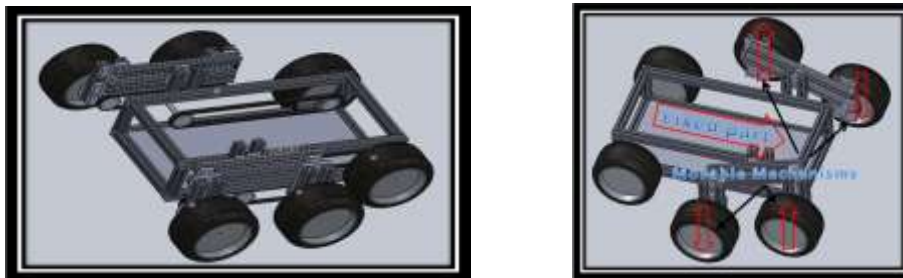
Fig. 8.1 3D robot structure with main tracking system depicted with climb accessories and mechanic displacement projected.
