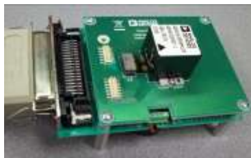
Fig 6.1 iSensor based in MEMS 3D level and acceleration [14].
