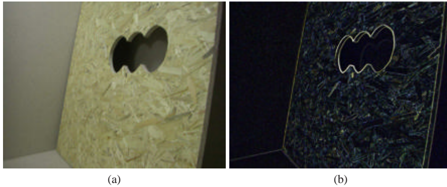
Fig. 6. Camera picture of three adjacent circles that are a possible location for victims. (a) Original camera image as input. (b) Same image after edge detection using the Sobel edge detection.
