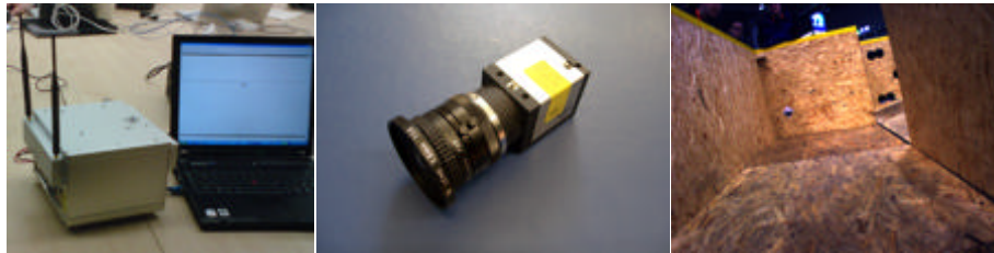
Fig. 4. Our mobile computing platform with CUDA capable GPU (left) and uEye camera (middle), and a picture taken by the camera at RoboCup German Open 2009 in Hannover (right).
