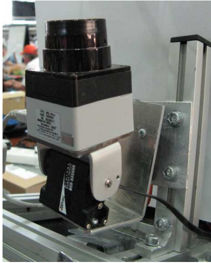
(a) The Hokuyo URG-04LX laser range finder (LRF), mounted on a rotation/tilt-unit.
