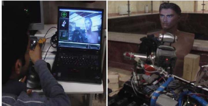
Fig. 5. Control Pack and Operator that's running the Robot and a sample of GUI
