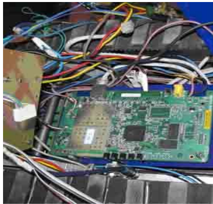
Fig. 3. Dlink Access Point Board
