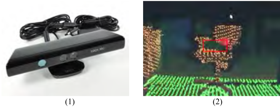
Fig. 8. Using (1) Microsoft Kinect for generating depth image to be used by the (2) hole-detection algorithm
