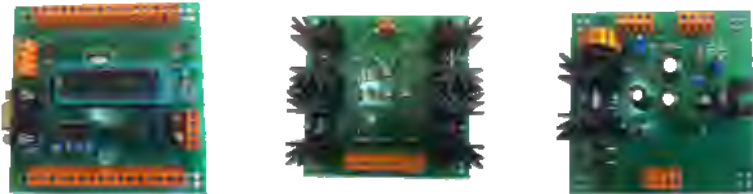
Fig. 12. The main control unit, h-bridge motor driver and the power unit of the robots.
