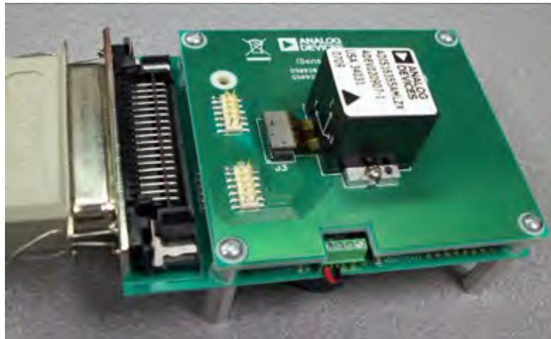
fig 6.2: iSensor based in MEMS 3D level and acceleration [14].
