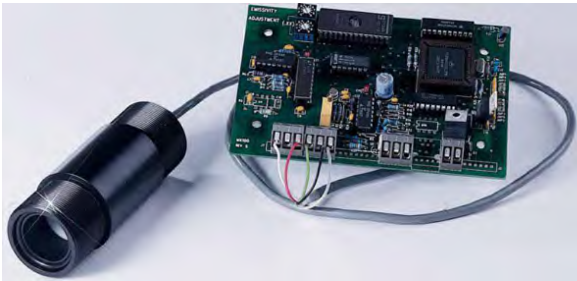
Fig.7.3 IR Sensor model OS65 used for body temperature measurement
