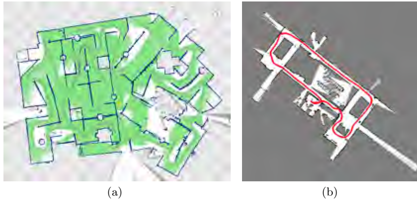
Fig. 2. Maps learned with the Hector SLAM system: (a): GeoTIFF map of the RoboCup 2010 Rescue Arena. The robot was carried through the arena by hand for this dataset, thus no odometry was available. (b): Larger scale mapping of a university floor with loop closing.
