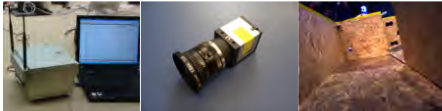
Fig. 4. Our mobile computing platform with CUDA capable GPU (left) and uEye camera (middle), and a picture taken by the camera at RoboCup German Open 2009 in Hannover (right).
