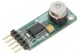
Fig. 11. The MLX90614 Infrared Thermometer
