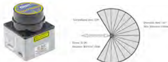
Fig. 6. Laser sensor (Hokuyo URG-04LX) and its field of view
