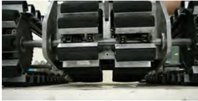
Figure 7- On flat surfaces supplementary tracks dose not hinder mobility
