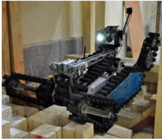
Figure 6- A pair of supplementary tracks under the main frame facilitates movement in uneven terrains
