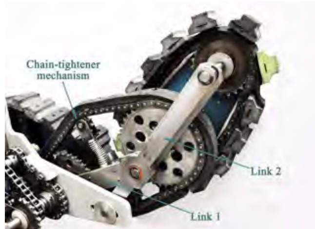
Figure 13- ADORA's Rear arm design
