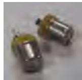
Fig. 5. RKRS custom thermal sensors with Perkin Elmer thermopile elements.
