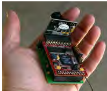
Fig. 3. Surveyor SRV-1 Blackfin controller with OmniVision OV7725 camera and Lantronix Matchport 802.11 b/g radio.
