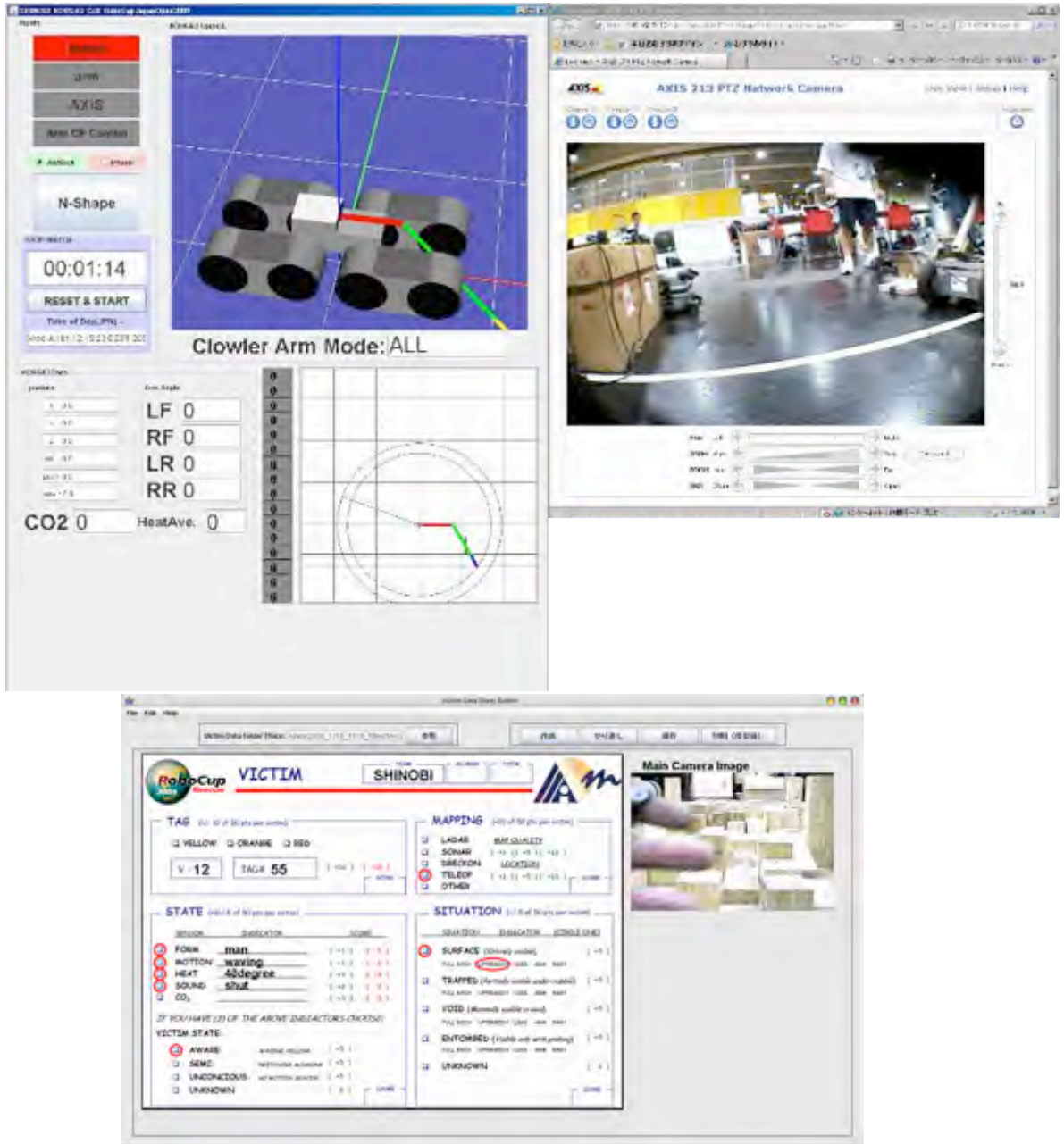
Fig. 9 automatic victim sheet print software (upper: input interface lower: output interface)
