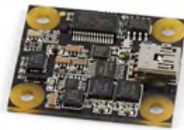
Fig. 1 Phidget 1056 - PhidgetSpatial 3/3/3 measures static and dynamic acceleration in 3 axes, magnetic field in 3-axes and angular rotation in 3 axes.
