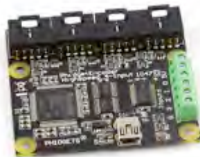
Fig. 2 Phidget 1047 - PhidgetEncoder HighSpeed 4-Input for the connection of up to four encoders.
