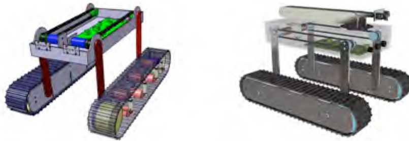
Fig. 4 The internals of the mechanism of the main body and the tracks and a photorealistic view of the robot.
