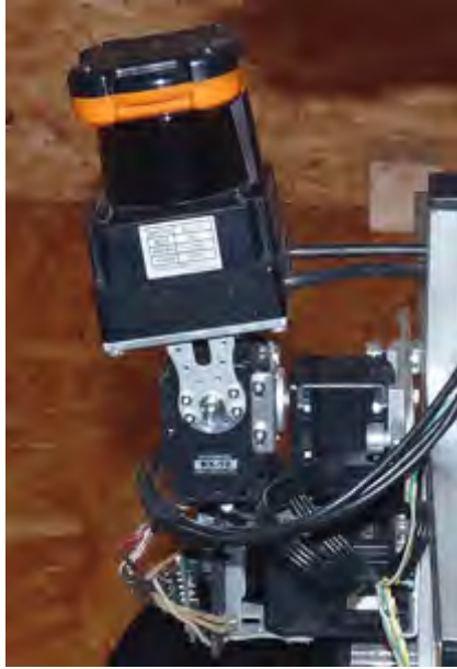
(a) The Hokuyo UTM-30LX laser range finder (LRF), mounted on a self-built rotation/tilt-unit.
