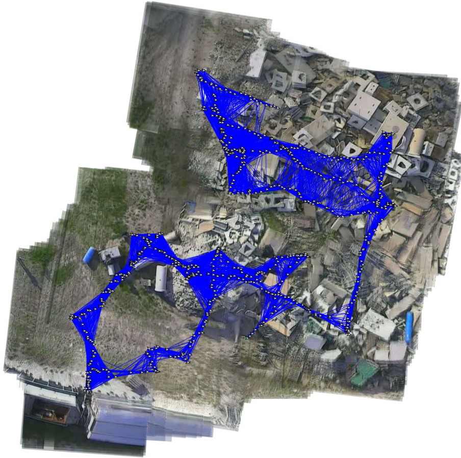
Fig. 5. An aerial map of a rubble pile at Disaster City made out of 630 video frames. Loop closing edges from a SLAM algorithm are shown (from [9]).
