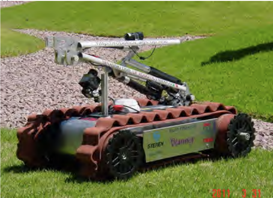
Fig. 4 Tracked wheel rescue robot IXNAMIKI ÖME: (a) design and (b) prototype.
