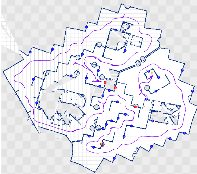
Fig. 2. Map learned using the hector_slam system at the final mission of RoboCup 2012. The robot started at the right middle position and autonomously explored the majority of the arena, finding 3 victims (red markers). The fourth victim was found using tele-operation on the last 4 meters of the travelled path. Blue markers indicate the positions of 35 QR codes that were detected autonomously by the robot.
