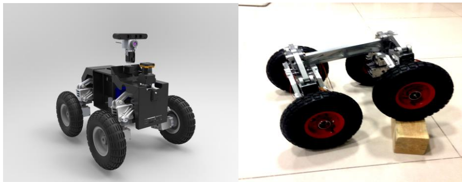
Fig. 11. Adrina's simulated and real mechanical platform
