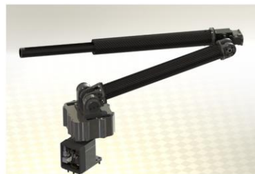
Fig. 9. New design of the 6 DOFs serial manipulator
