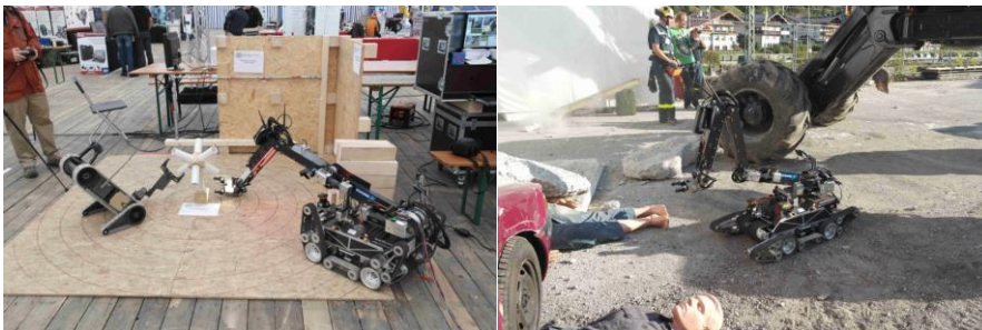
Figure 2: Pipe inspection with MARK and iRobot 310 SUGV and Outdoor training at EURATHLON 2013
