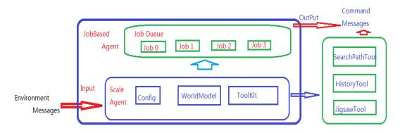
Figure.1 Software Architecture
