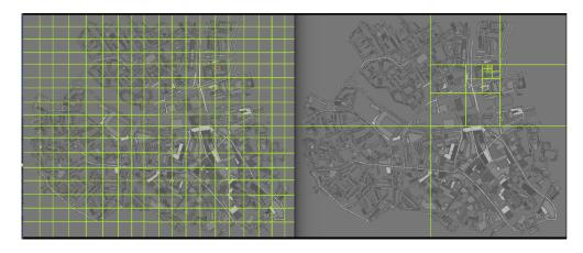
Fig 1. Comparison of Cellularization and Quadtree Cellularization - Eindhoven
