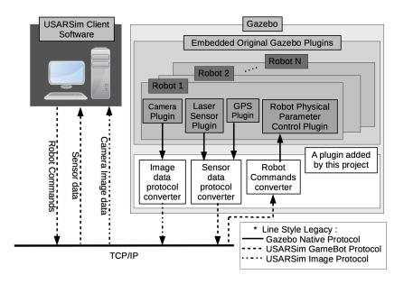
**Fig. 1.** Diagram of our prototype simulator with Gazebo. At right middle of the diagram, white blocks are our added plugin software in Gazebo. The plugin translate bidirectionally USARSim commands and Camera images and Sensor data between USARSim protocol(GameBot) and Gazebo Native protocol(Topic).
