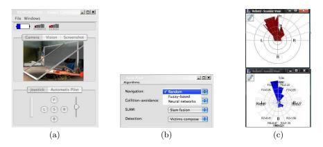
**Fig. 3.** Screenshots of the control system: a) The robot individual controller: icons allow easy and quick identification of battery and communication level with other robots; b) Algorithms loaded as plugins can be selected by operator in running time; c) laser scanner and sonnar viewers.
