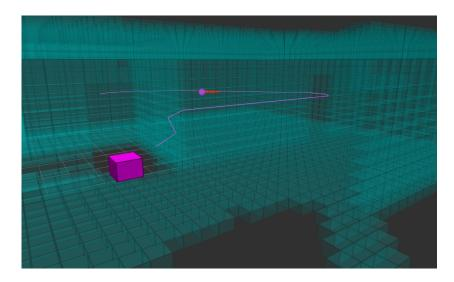
Fig. 7. A calculated path between a robot and its goal by  $\mathrm{A}^*$
